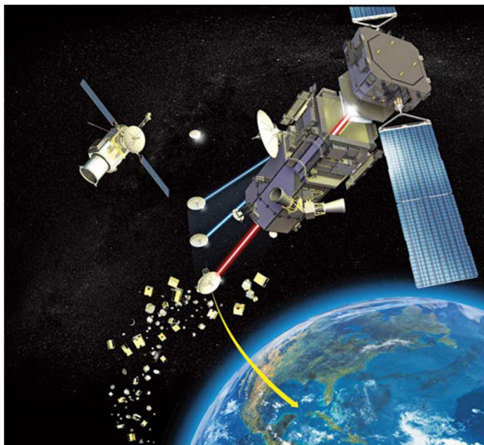
Micro Remover tether-extensible gripper with foldable arms, JAXA.
