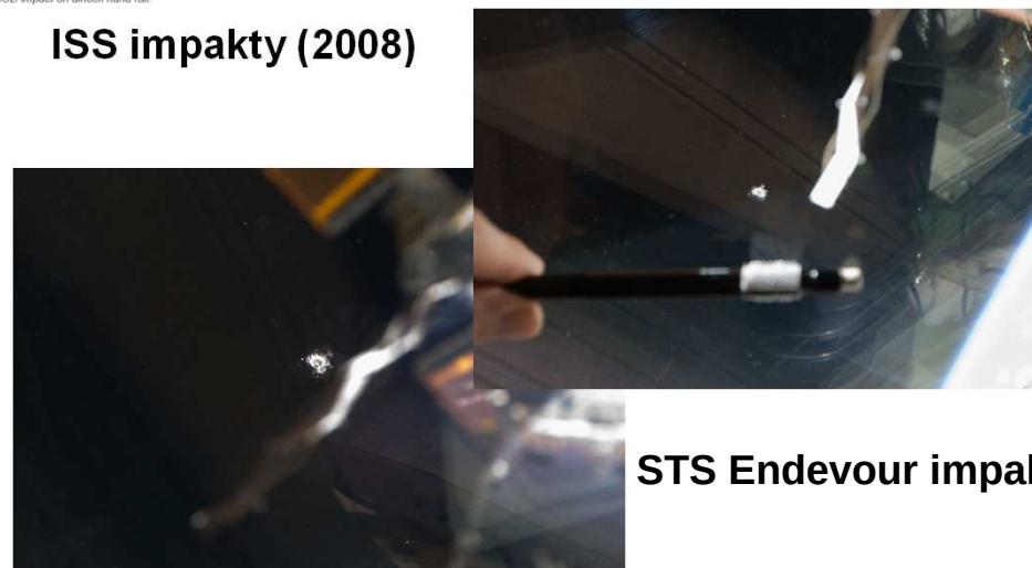
Figure 2. Detail of MMOD impact on airlock hand rail.
